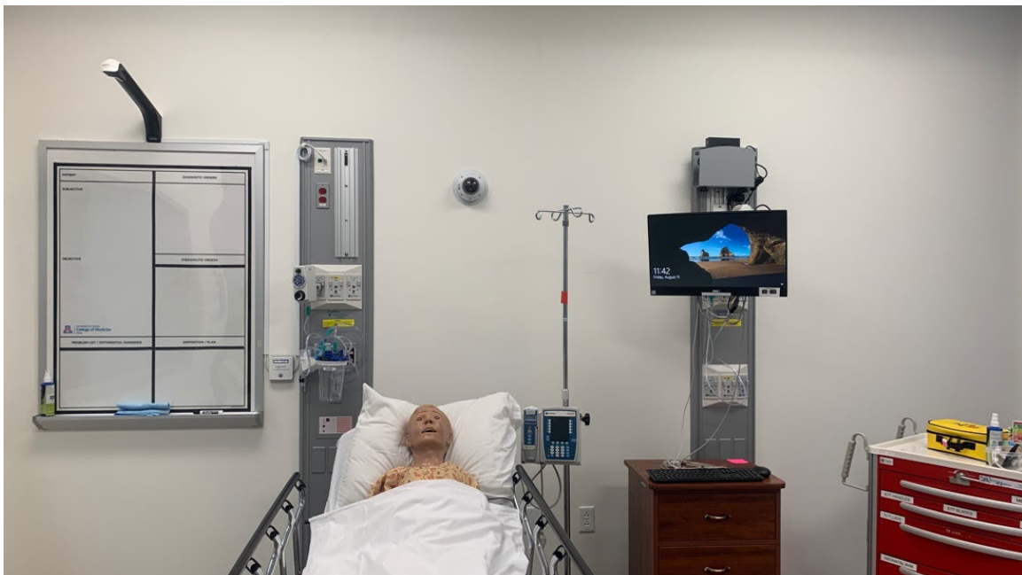
Figure 2.2: The start/end session button (B) turns on the telescopic camera (A) that captures the information on the whiteboard overlay template (C).
